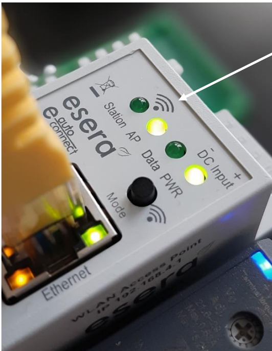
Access Point is activated
